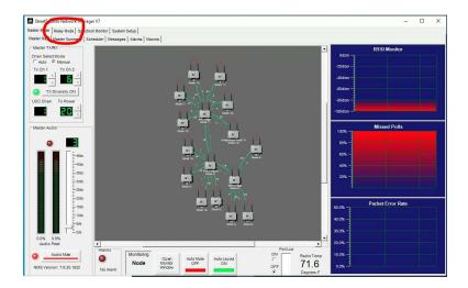
This will switch the Primary Fixed Master into Relay mode. However, the Fixed Master must be manually configured to receive the specific channel that the Secondary Master Transmitter is transmitter is transmitting on.
