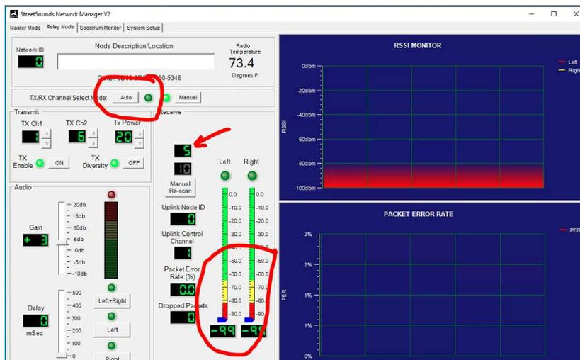
3. Turn on the Secondary Fixed Master Transmitter to the selected channel. To do this you may need to temporarily connect the NMS to the Secondary Master to properly configure its transmit channel.
