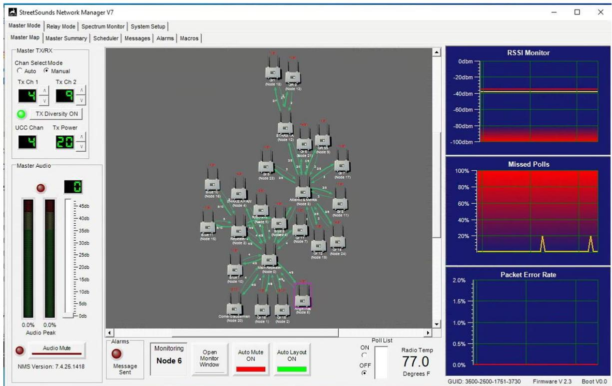
StreetSounds networks can operate with or without the NMS (“Managed” or “Unmanaged” network). However, when there is no NMS, there is no visibility into the network for troubleshooting or control.
