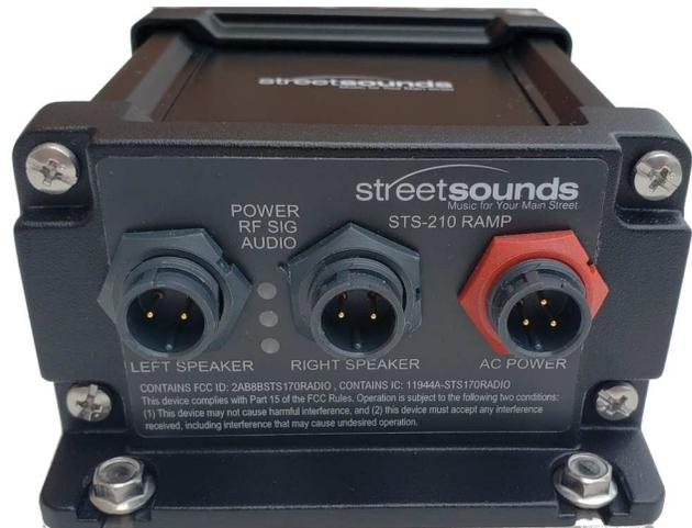
The StreetSounds® “RAMP” is a combination digital Radio (900 MHz) plus a 2-channel 20 watt class-D audio amplifier, housed in a rugged, weatherproof aluminum enclosure built to withstand harsh, outdoor environmental conditions in permanent installations.
