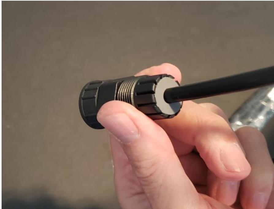
**Tighten the Sealing Nut**
