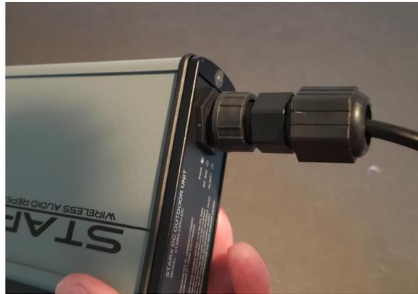
The KIT-ST5-200-FMST also includes a weather boot to protect the outdoor end of the RJ45 cable from the elements. IF NOT ATTACHED, THE RJ45 CONNECTOR WILL DETERIORATE OVER TIME AND CAUSE ISSUES WITH CONNECTIVITY BETWEEN IDU AND ODU. FAILURE TO ATTACH THE WEATHER BOOT WILL VOID THE WARRANTY. Please see detailed assembly instructions at the end of this document.
