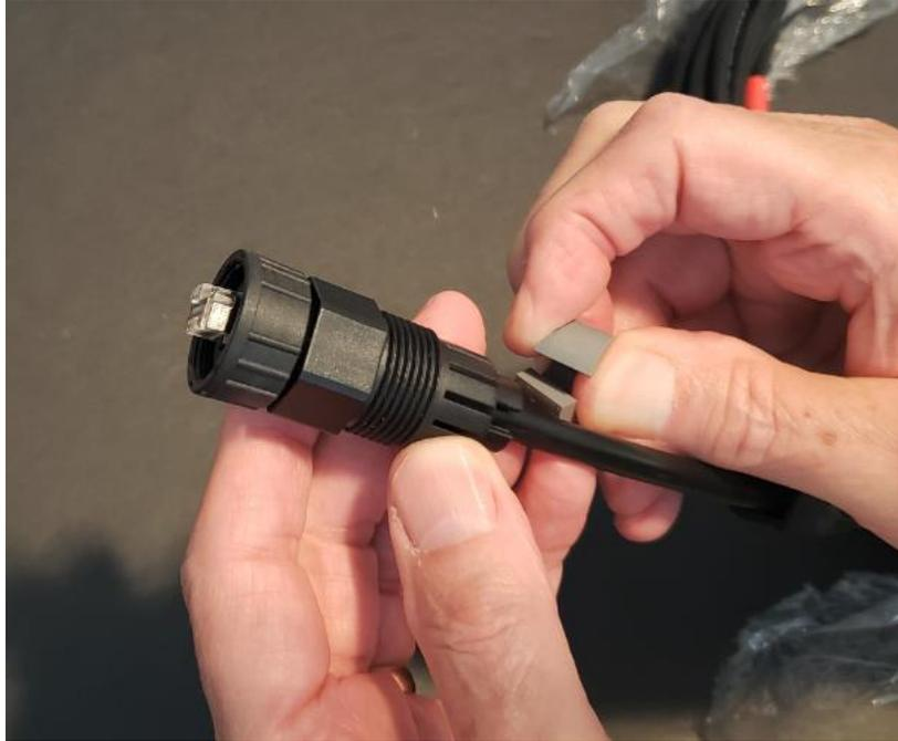
Push the seal upward into the housing so that it is fully inside the housing.
